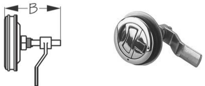
Hatch fastener #43.1953 (set) Includes: Cam and strike. Dimension A = 2 25/64" Dimension B = 3 3/4" Cut hole 2" diameter Standard spring loaded strike included.
