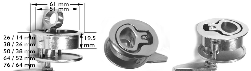
thread allows for 12 mm play #43.5205 Locking hatch pull with 1/8" compression when locking lever Order with cam to fit. More info see page 4-3-3 l
