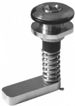
43.1026; 40 mm outside diameter, 24 mm inside diameter. For up to 3/4" material thickness. Cam reach: 2 3/4" By turning key the cam tightens against the strike plate
